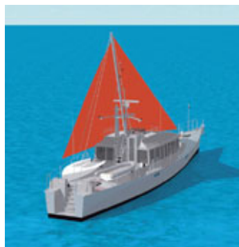
MARATHONER: Everything about the Dashew 83 aids in her ability to go long distances with maximum seaworthiness, including a fallback emergency sail raised off the boom.
